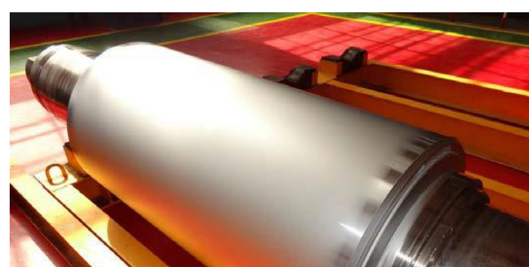
Roller after EDT process with a smooth and homogeneous roughness
